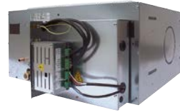
OBU10 Omnibus card with Modbus for brushless motors
