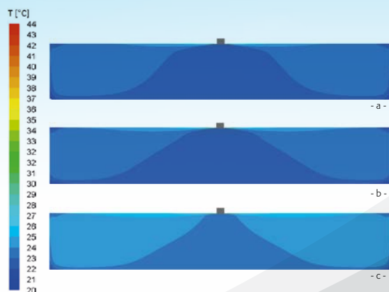
Fig. 4a UCS600: Distribution of air temperature [°C] in winter mode, on a vertical plane that divides the room in two parts, at MIN (a), MED (b) and MAX (c) speed.
