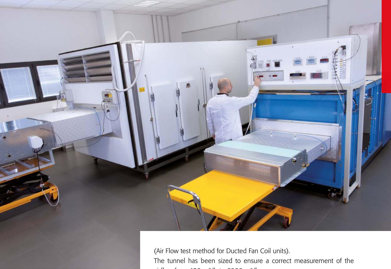
(Air Flow test method for Ducted Fan Coil units).
