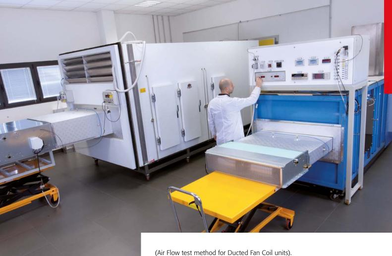
(Air Flow test method for Ducted Fan Coil units). The tunnel has been sized to ensure a correct measurement of the airflow from 120 m<sup>3</sup>/h to 6000 m<sup>3</sup>/h.
