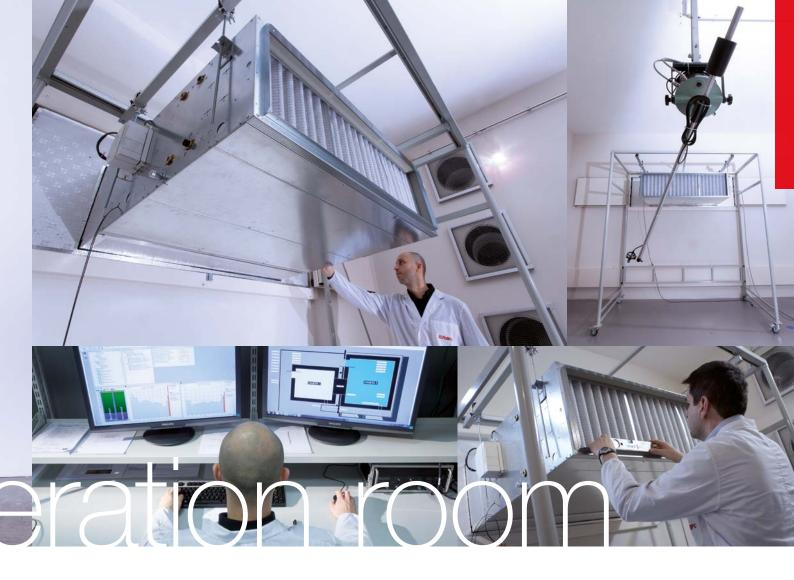
The two reverberating rooms have different dimensions: 84 and 127 m³ respectively and are connected each other by an air duct.
