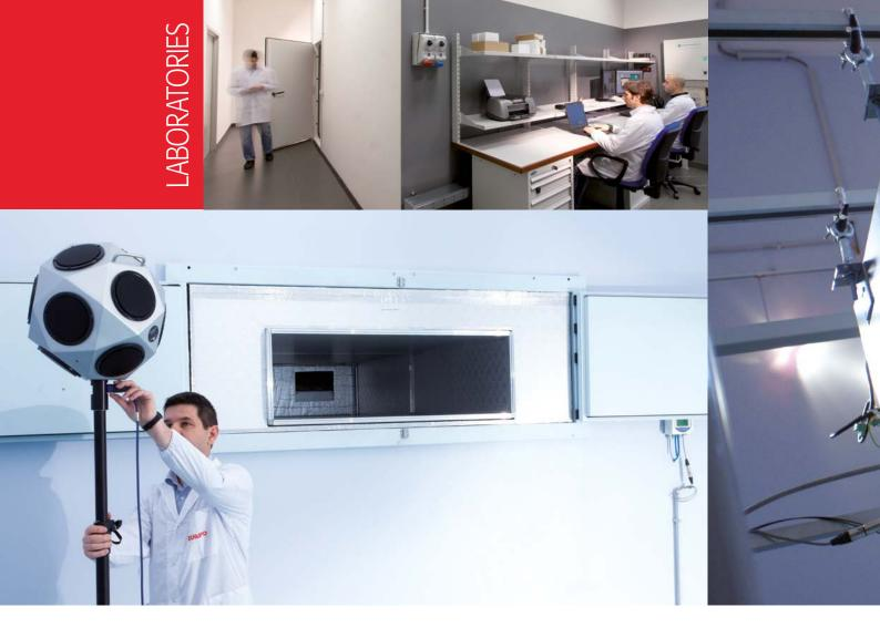
The purpose of the larger reverberation room is to perform acoustic tests in order to measure the sound power level of sources operating either in the same environment (for example fan coil units) or in a separate room (the smaller reverberation room), but having direct acoustic input in the measuring environment (ducted units).
