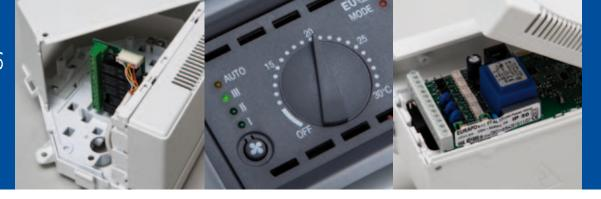
The **heart of the system** is the **POWER OMNIBUS** card: this highly-flexible piece of hardware is installed in the terminal unit and enables the firmware to be upgraded **through a serial port**. It can easily be programmed and configured to requirements by the user and by the installer to the type of system being installed.
