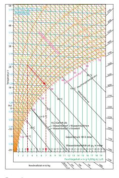
**Example:** Air at 21 °C / 3 g/kg is humidified to 7 g/kg.
